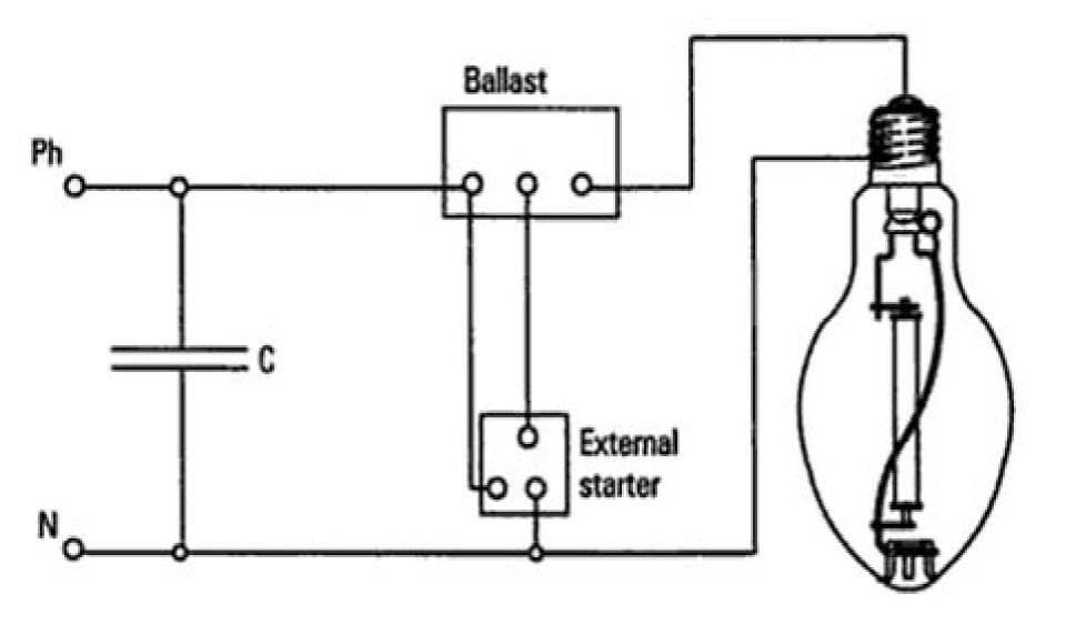
Figure 2 SON - starting method circuit diagram
