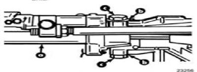
**Power Steering Units Secured With Pivot Bolts**
