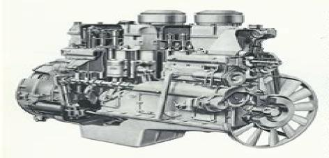
680 MK.II DIESEL ENGINE (STANDARD)—This engine is a 200hp unit for high performance applications. It is generally similar to the standard engine described in this specification.
