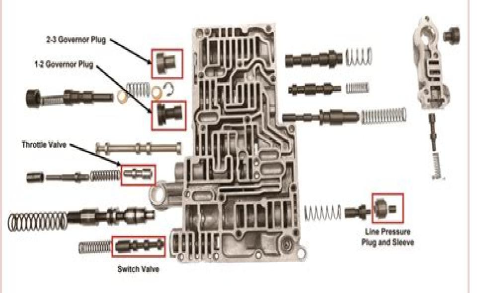
Figure 1: On a disassembly inspection, always inspect these valves and valve bores!
