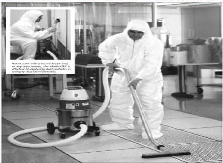
The Model CRV is designed for use in Class 1 Class Room environments to reduce the incidence of airborne contominants.
