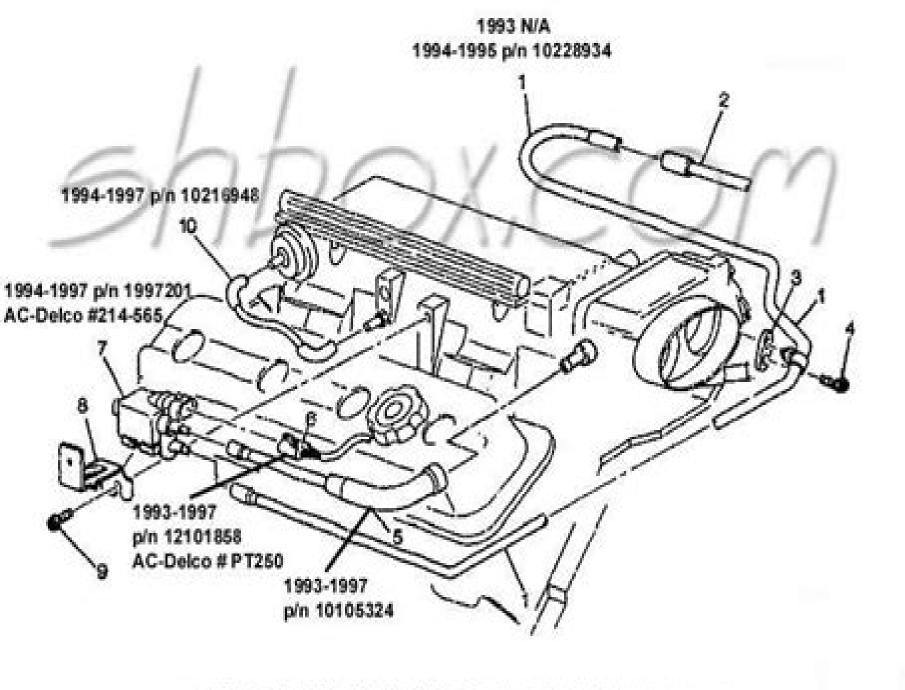
1993-1995 F VAPOR CANISTER LINES & VALVE (LT1/5.7P)
