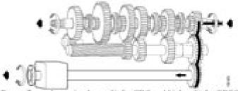
Power flow when using low split for GRS and high split for GRSO.
