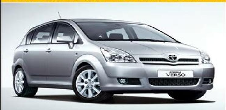
MOTORES: 2.0L Turbo Diesel (1CD-FTV) -1.8L (1ZZ-FE) - 1.6L (3ZZ-FE)
