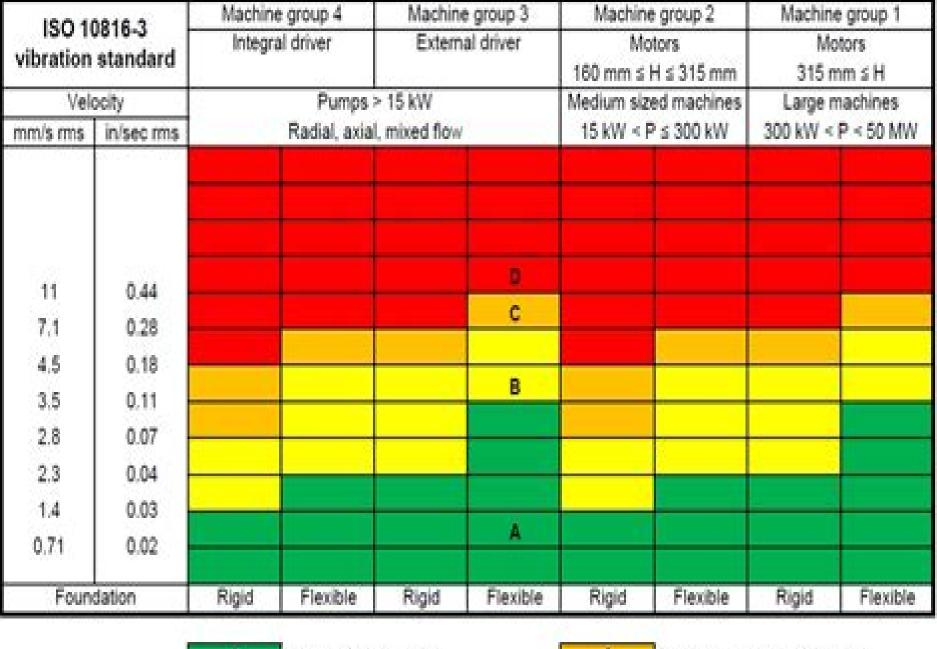
B Unlimited long-term operation allowable D Vibration causes damage
