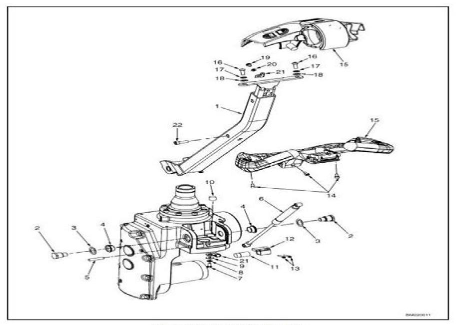
Figure 3. Control Handle Assembly
