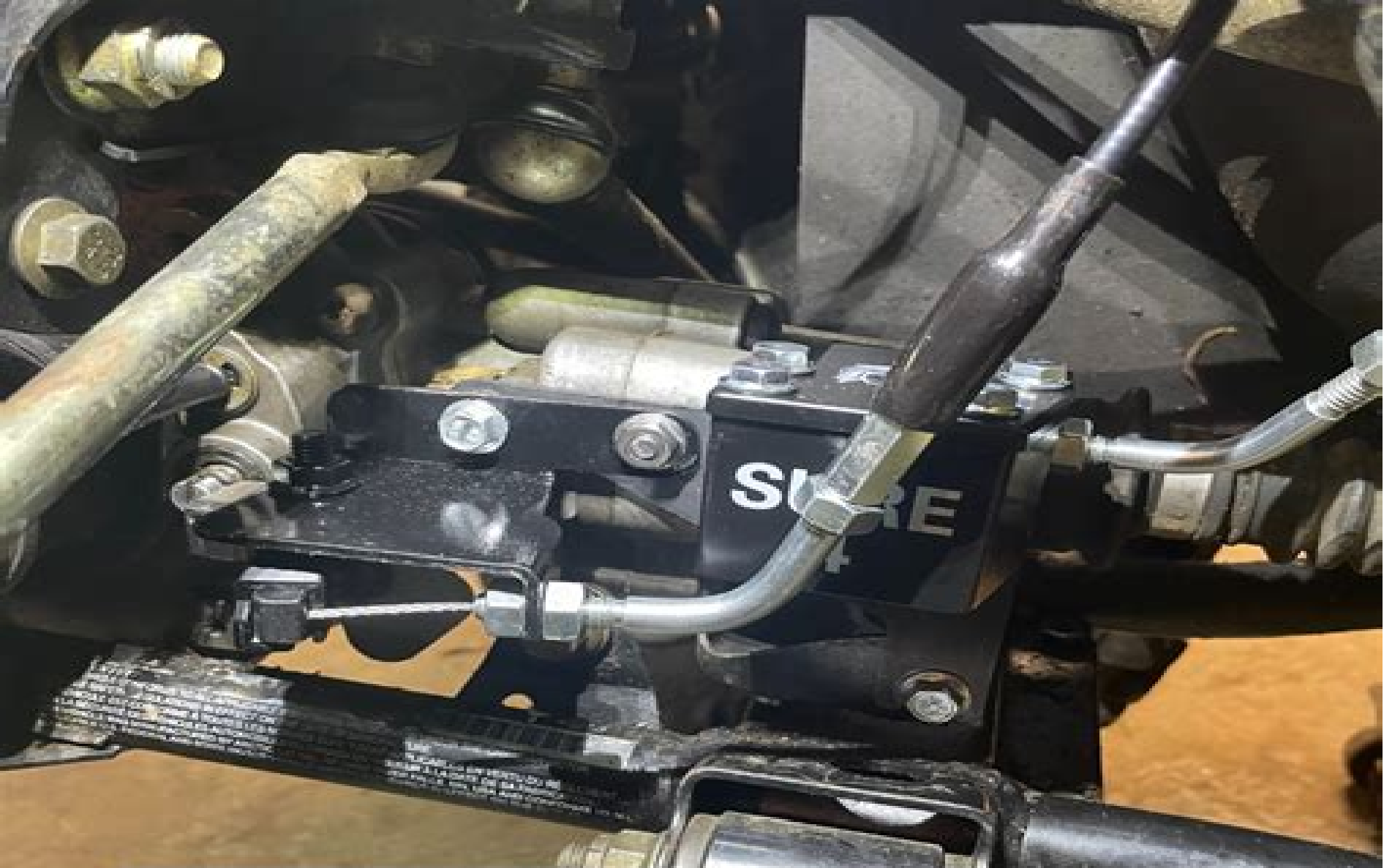
*This is what your Sure 4 acuator should look like once fully installed*
