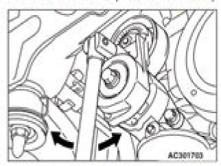
Securely insert the spindle handle or ratchet handle with a 12.7 mm insertion angle into the jig hole of the auto tensioner. Turn the auto-tensioner to the left and right to check and see that there is no threading. Measure the drive belt tension vibration frequency by the following procedures:
