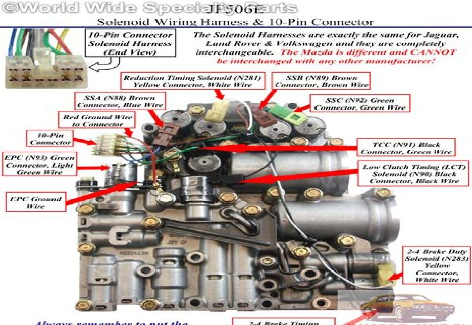
Always remember to put the EPC Ground Wire & the Red Ground Wire from the 10-Pin Connector under the bolts shown!
