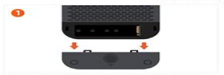
Remove the SSD enclosure cover on the bottom of the stand.
