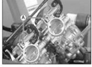
Hold the starter plunger springs compressed, and free the choke cable lower ends [A] from the plungers [B].
