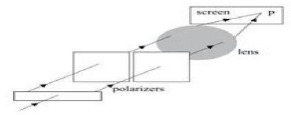
A lens brings the light to focus at point P on a screen. The lens does not introduce any additional path difference.
