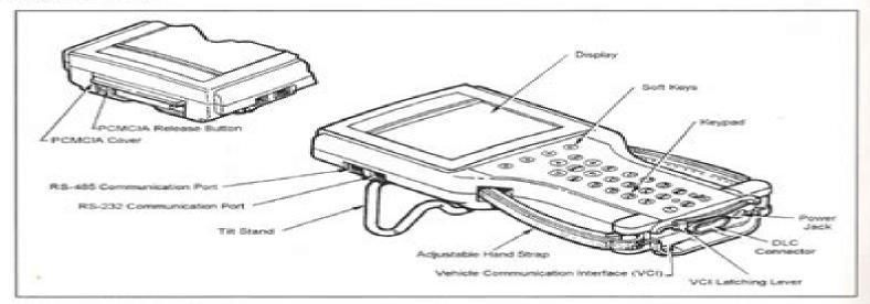
Tech 2 is a hand held diagnostic computer, designed specifically to help you diagnose and repair problems with a whole range of complex electronic systems. When Tech 2 is attached to a vehicle, it guides you step-by-step through each of its programmed test procedures. Tech 2 functions are accessed through its keyboard, commanding it to:
