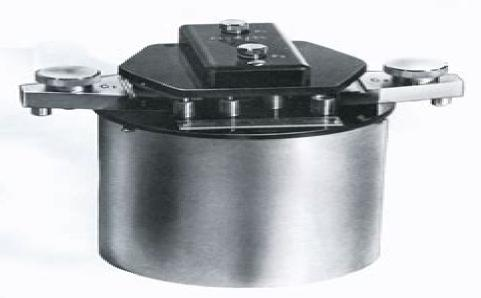
Temperature Coefficient Within ±5 ppm per degree centigrade at 25 C. A table is provided with the standards giving corrections from 25 C for every 0.1 C from 20 to 30 C. Corrections are given to the nearest 0.1 ppm. Alpha, beta, and peak are also given.
