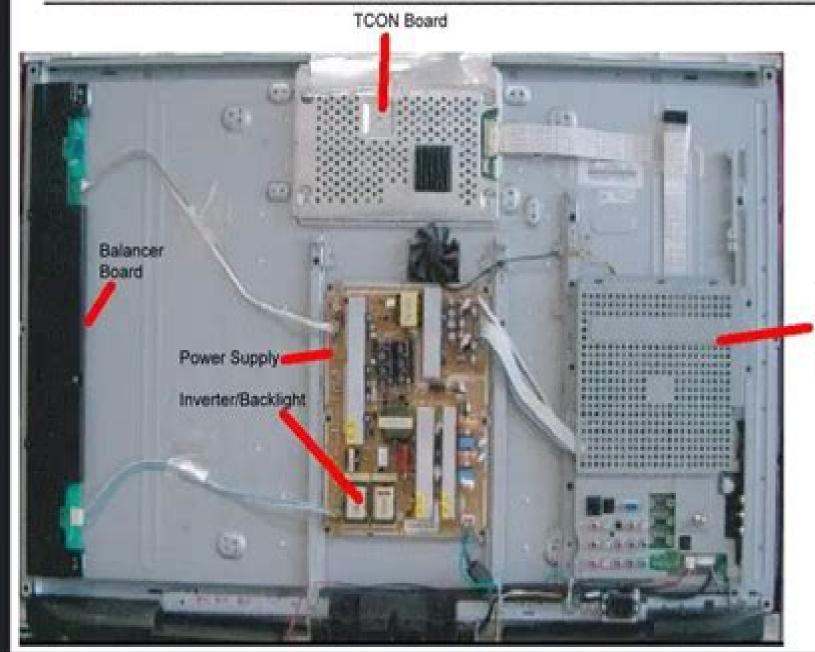
Main Board -Video/Audio Input Switch Microprocessor
