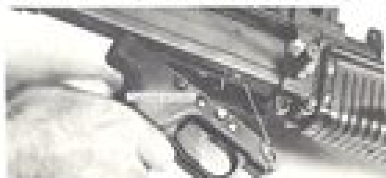
Figure 13. — Removing the Trigger Housing.
