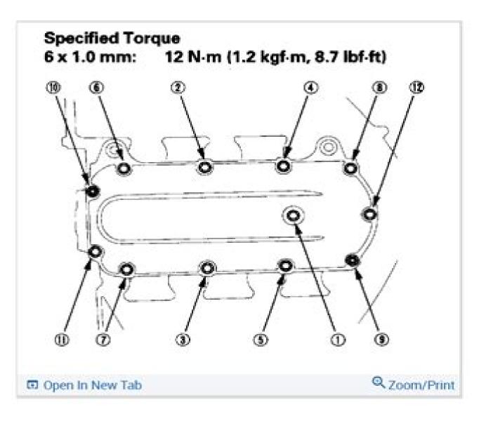
Install the upper cover. Tighten the bolts and nuts sequentially in two or three steps.
