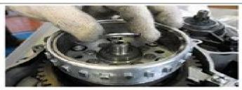
Fit the tool and pull out the rotor.
