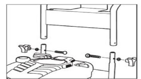
Step 1 Attach the handle to the frame of the pressure washer. Align holes, insert bolt, and tighten with knob.
