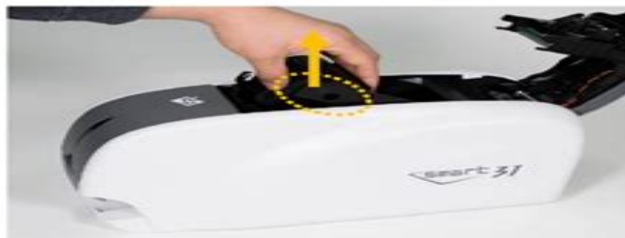
Figure 10 Take out the ribbon cartridge
