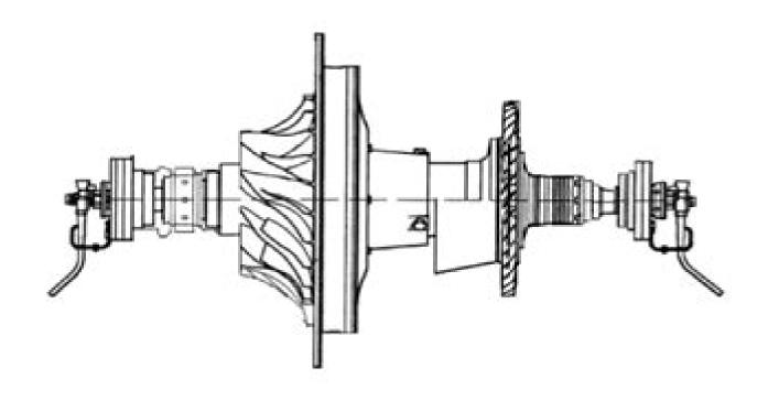
Rotor complete with bearings and oil pumps
