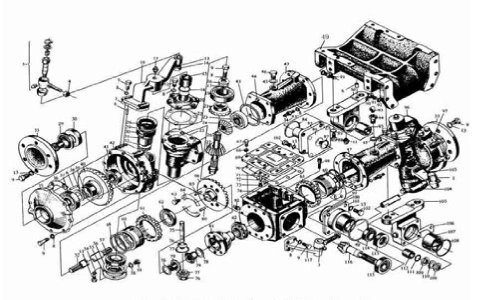
Fig. 3-A Front Axle For Hydraulic Steering
