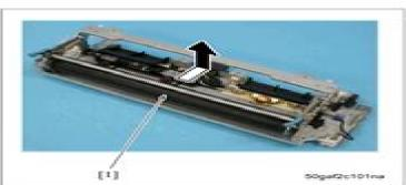
A 13. Remove the fusing pressure roller [1].
