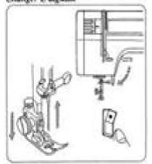
Raise the needle by turning the balance wheel toward you and lower the preser foot.
