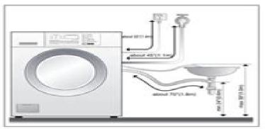
Properly securing the drain hose will protect the floor from damage due to water leakage.
