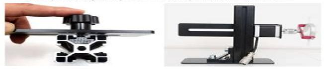
B. Use an Allen wrench to screw M8 with washer
