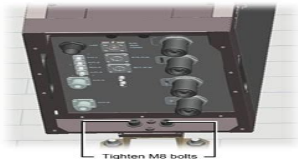
Figure 16: Tighten the Screws at the Bottom of RU
