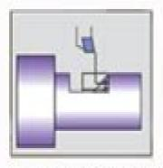
Machining in counter direction
