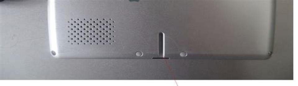
Mount is for Navman GPS with such mount socket.
