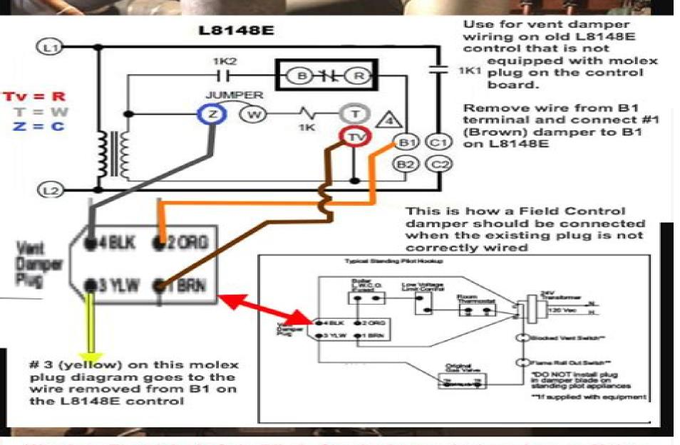
Warning Electricity is ColorBlind. Check wire terminal numbers on Molex connector 1,2,3, and 4 to determine actal conector wire colors on your damper wire harness
