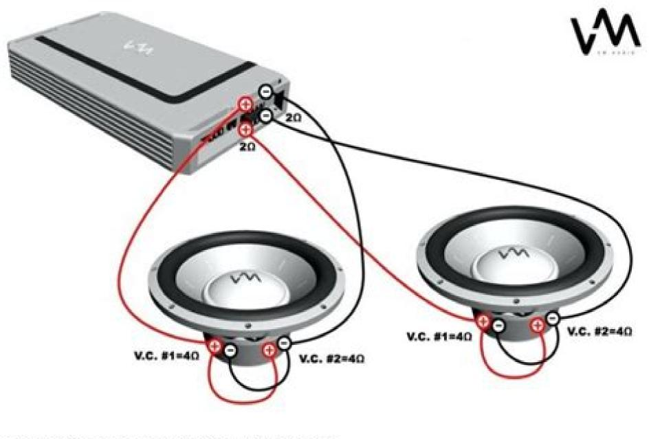
TWO 4Ω DVC SUBS, BRIDGED 4-CHANNEL AMP: 2 X 2Ω LOAD
