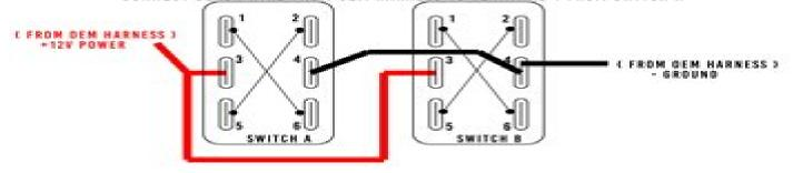
STEP 3: CONNECT TERMINAL 5 FROM SWITCH A TO RED/BLUE STRIPE WIRE CONNECT TERMINAL 6 FROM SWITCH A TO GREEN/BLUE STRIPE WIRE CONNECT TERMINAL 5 FROM SWITCH B TO GREEN/WHITE STRIPE WIRE CONNECT TERMINAL 6 FROM SWITCH B TO GREEN/WHITE STRIPE WIRE
