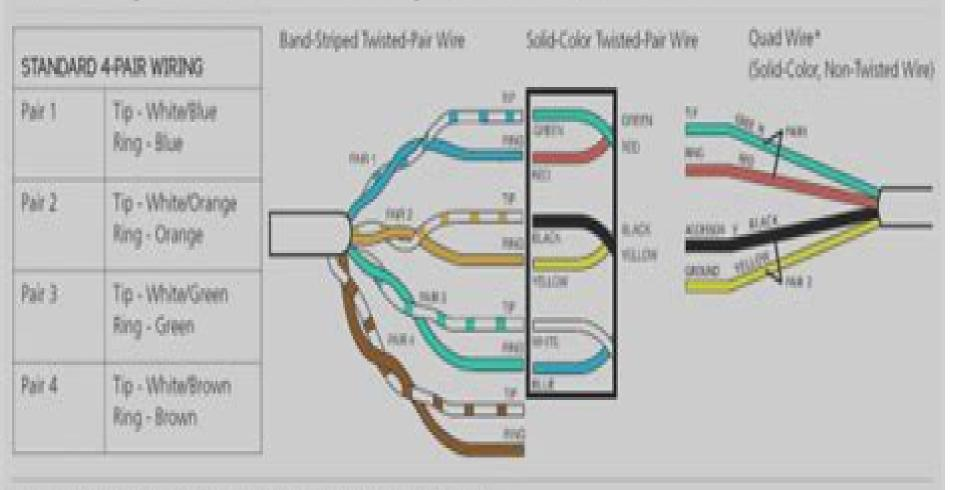
For 6-wire jacks use pair 1, 2 & 3 color codes. For 4-wire jacks use pair 1 & 2 color codes.
