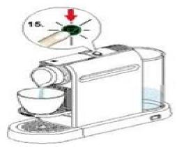
Rinse coffee machine by pressing any button and wait until water tank is empty.
