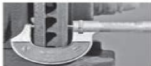
Measuring brake rotor wear. 00.04 Maintenance
