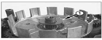
Take the supporting disc • and the outer clutch hub together with the bearing off the main shaft.
