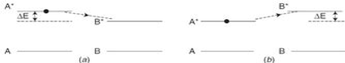
Figure 11.1 (a) Exothermic and (b) endothermic excitation from atom A to atom B.
