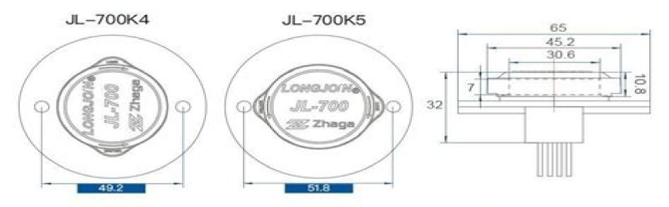
\* The Zhaga receptacle to be enabled installed onto a NEMA opening.
