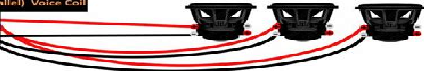
3 Sub, Single (Parallel) Voice Coil
