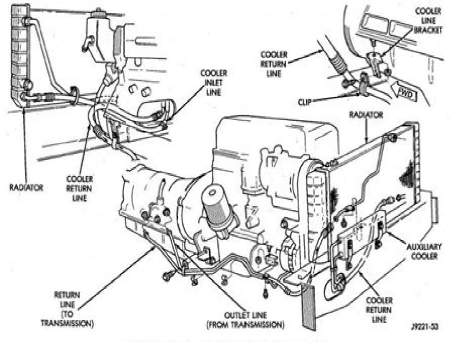
Fig. 48 Auxiliary Cooler Mounting (Left Hand Drive)
