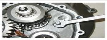
Use rubber bands to tie down the transmission shaft unit and extract it.
