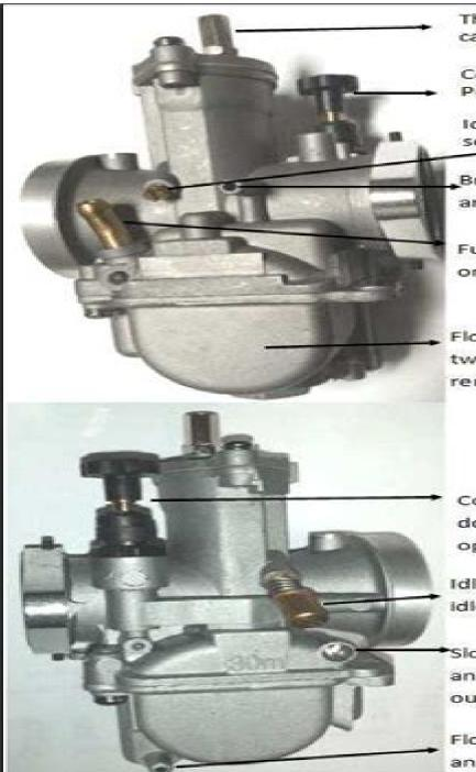
Throttle cable adjuster, use to adjust free play in cable housing.
