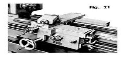
A special carriage, Figure 21, is provided with the cross slide located at the left of the carriage wing. This allows the operator to place his tools to takefull advantage of the gap. An extension rest (optional equipment) facilitates even fuller use of the gap.
