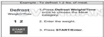
NOTE: After you press START/Enter, the display counts down the defrost time. The oven will beep once during the defrost cycle. At this time, open the door and turn, separate, or rearrange the food as needed. Remove any portions that have thawed, then return the frozen portions to the oven and press START/Enter to resume the defrost cycle. The oven will not stop following the beep unless the door is opened.
