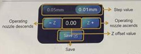
After the machine stops, adjust the offset value of Z axis in order to adjust the stance between nozzle and hot bed.
