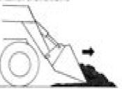
Spread det by driving forward with bucket filled down and remail off the ground.
